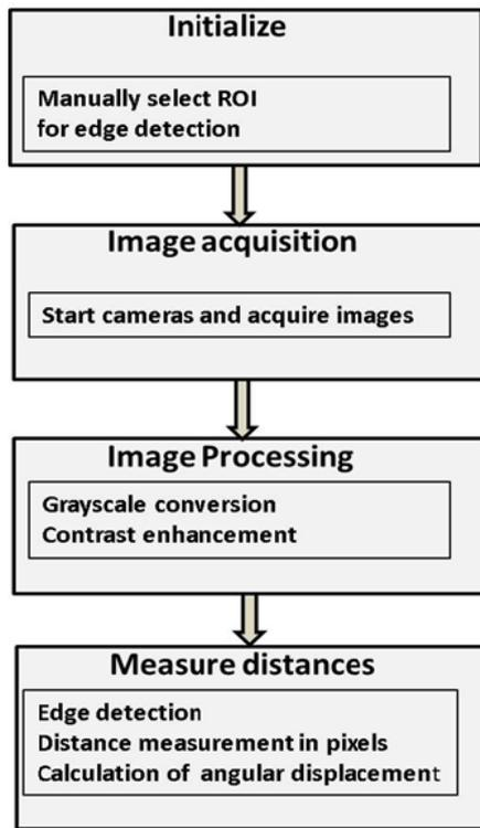
Figure 4: Labview algorithm flowchart.
