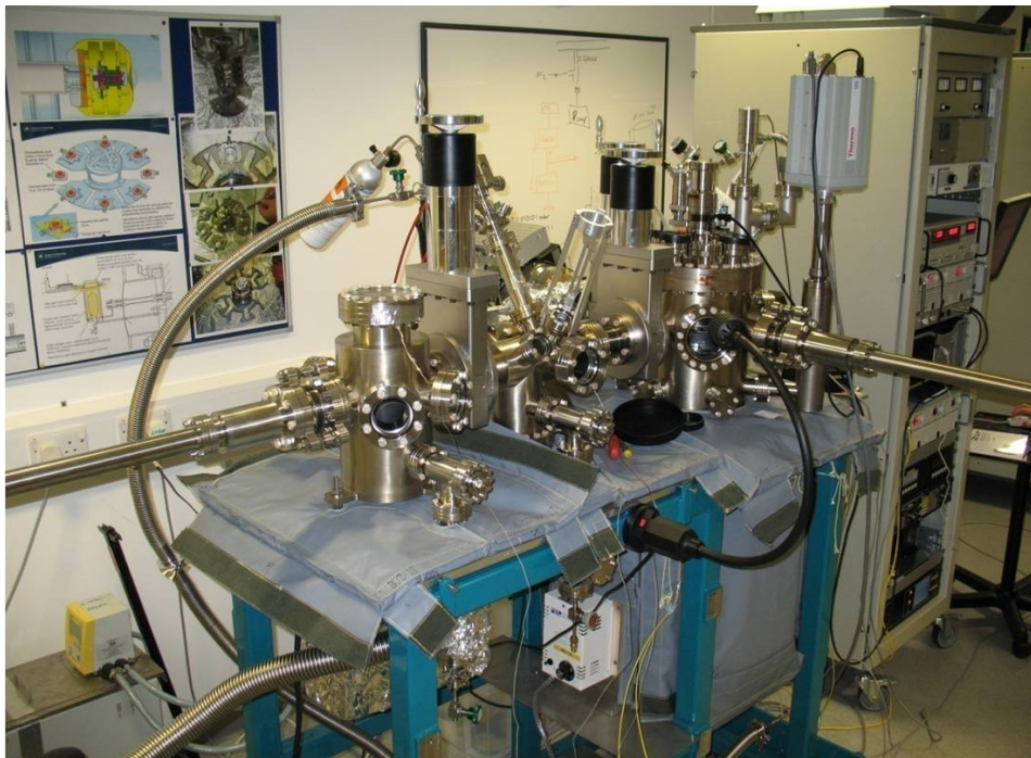
Figure 7: The assembled photocathode preparation facility.
