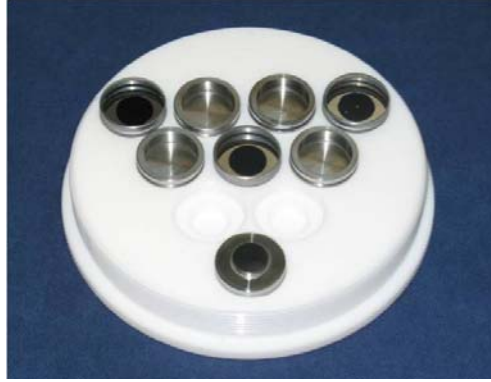
Figure 5: GaAs photocathodes on molybdenum substrate
