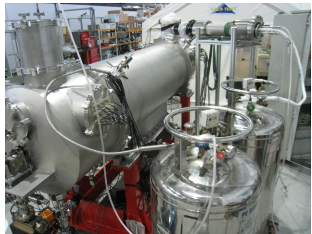
Figure 2: Fully assembled cryomodule undergoing Qualification tests.
