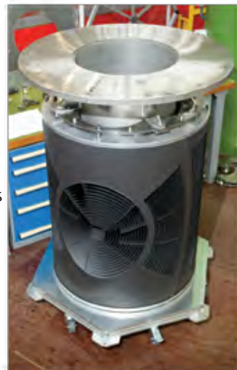
The novel ^{10}\text{B} -coated radial collimator assembly before installation on Polaris
