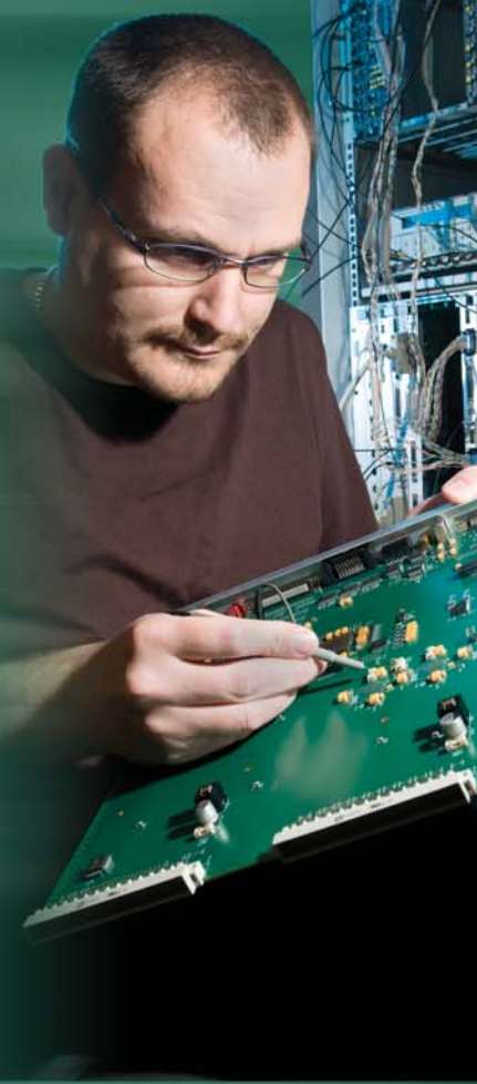
Right: Matt Roberts (ISIS) testing the new TDC card for the muon suite of instruments.
