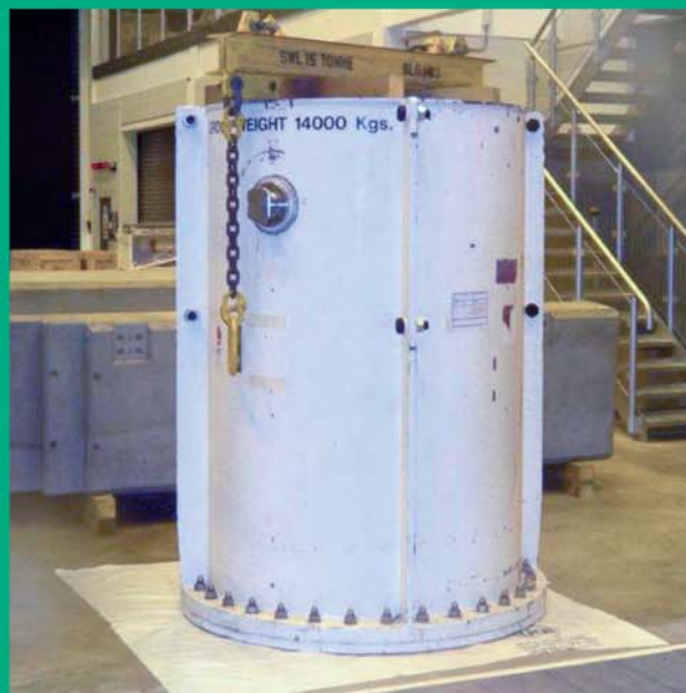
The ISIS Target Transportation flask loaded with a spent target ready for transportation to Sellafield.
