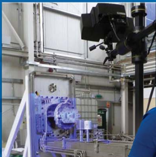
Left: Scanning the mock-up of the TS-1 target, with CAD comparison of the scanned data below.
