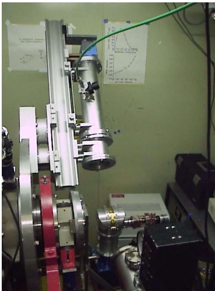
Fig. 2. The diffractometer inside the hutch with the cryostat mounted on the \omega -circle. The photograph was taken from above the incident beam pipe.
