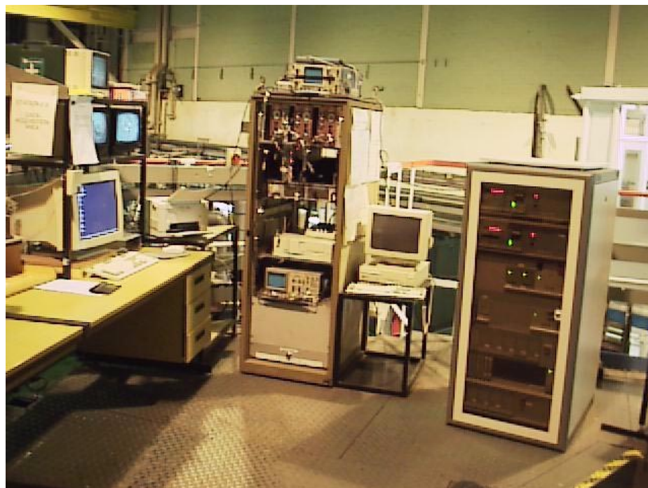
Fig. 3. The control computer, electronic racks, McLennan system and TV monitors on the gantry.
