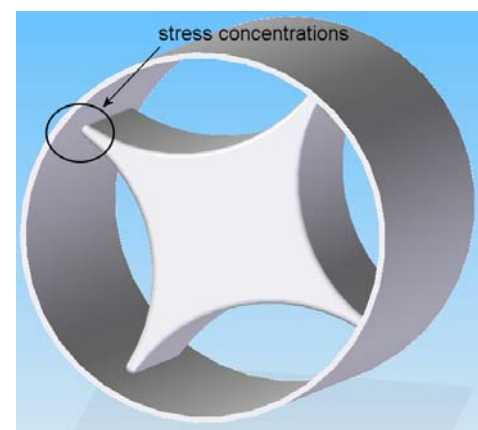
Figure 3.3.43 Target segment with rounded fin joints
