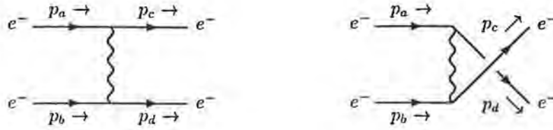
Figure 4.2 Lowest order Feynman diagrams for electron-electron scattering.
