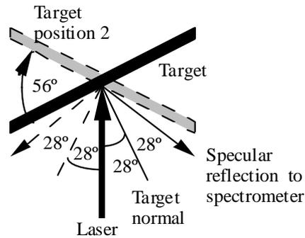
*Figure 4. Schematic of the targets angular position with respect to the incident laser beam. The black target and solid lines represent the normal target position 1, with the spectrometer in the specular reflection direction. The grey target and dashed lines represent target position 2 with the angle of incidence, at  $28^\circ$ , and the spectrometer position remaining the same, but with the specular reflection direction being  $112^\circ$  from the previous direction.*
