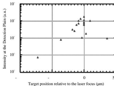
Figure 2. Third harmonic intensity at the detector, as a function of target position relative to the laser focus
