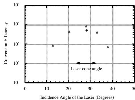
Figure 6. Conversion efficiency into the third harmonic versus angle of incidence of the laser with respect to the target normal. The triangles represent the average of at least 2 data points, with the target in position 1. The circle represents emission collected with the target in position 2, see figure 4. The black arrow represents the angular divergence of the laser
