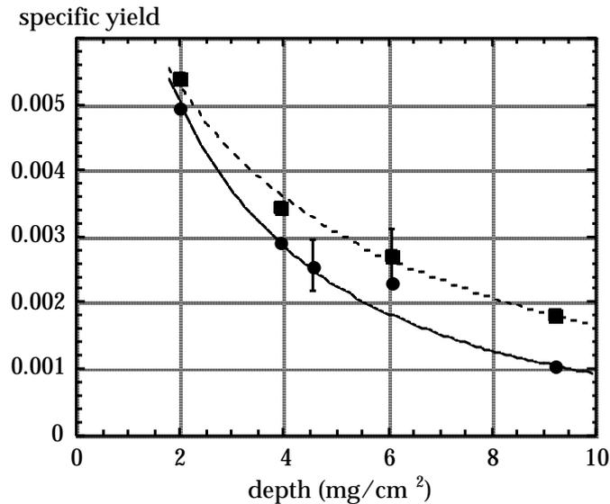
**Figure 5.** Specific k-alpha yields from uncompressed (●) and compressed (■) as a function of depth of the buried fluor layer. The continuous line is due to the model of Harrach and Kidder for a curvilinear range of  $2.7 \text{ mg cm}^{-2}$  and the broken curve for a range of  $5.8 \text{ mg cm}^{-2}$ .
