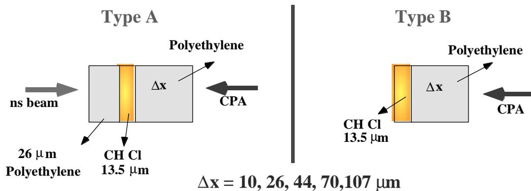
**FIGURE 2.** type of targets used in the experiment.
