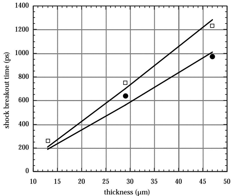
**Figure 4.** Shock breakout time for three different thicknesses of plastic target. The open squares are the experimental values for an irradiance of  $1 \times 10^{15} \text{ Wcm}^{-2}$  and the filled squares are for an irradiance of  $1.5 \times 10^{15} \text{ Wcm}^{-2}$ . The continuous lines are the predictions from the MULTI code for the respective irradiances.
