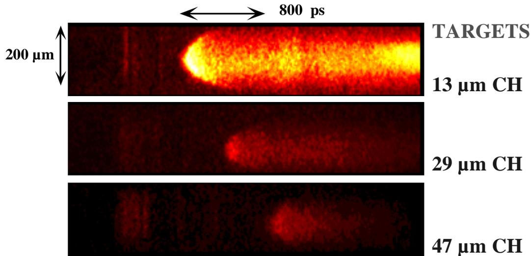
**Figure 3.** Streak camera images of shock breakouts with targets of different thickness.
