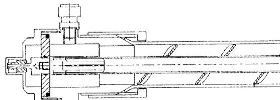
Figure 3: Cross section of BLM (70 MeV system).
