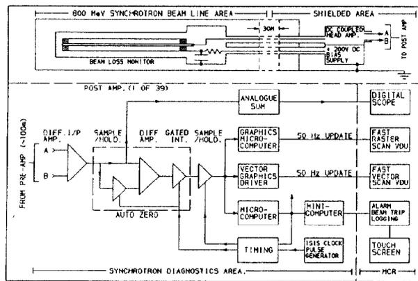
Figure 6: 800 MeV synchrotron system schematic
