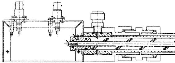
Figure 5: Cross section of BLM (800 MeV system).
