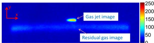
Figure 2: Beam profile from the supersonic gas-jet monitor.
