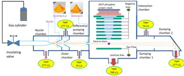
Figure 1: Schematic diagram of the supersonic gas jet setup.
