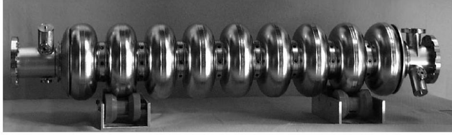
Figure 2.3: Photograph of a TESLA cavity. Adapted from [23].
