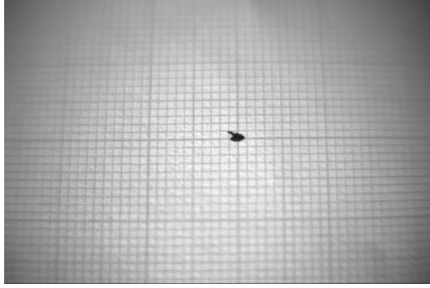
Figure 3.5: An image of a reference millimetre paper placed on the surface of the scintillator.
