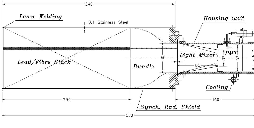
Figure 2: Schematic drawing of a hadronic module.
