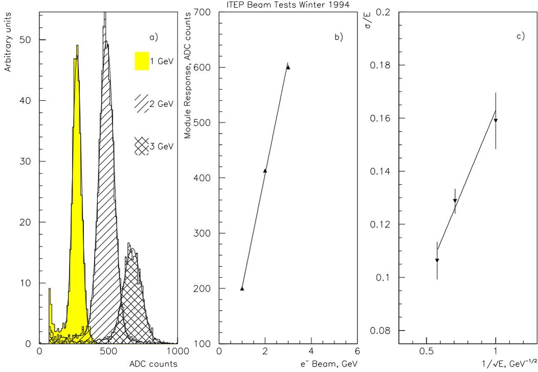
Figure 4: Response of the hadron module to the ITEP electron beam: a) signal spectra in ADC counts, b) linearity of the response, c) fit to the electromagnetic resolution.
