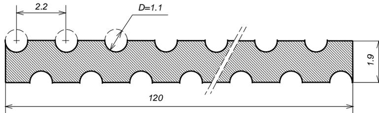
Figure 3: Profile of the lead sheets that were stacked to form the hadronic modules.
