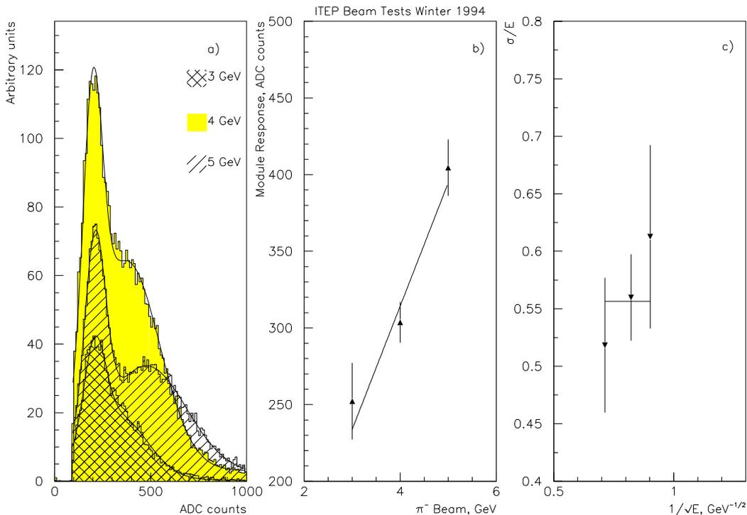
Figure 5: Response of the hadron module to the ITEP  $\pi^-$  beam: a) signal spectra in ADC counts, b) linearity of the response, c) the hadronic resolution.
