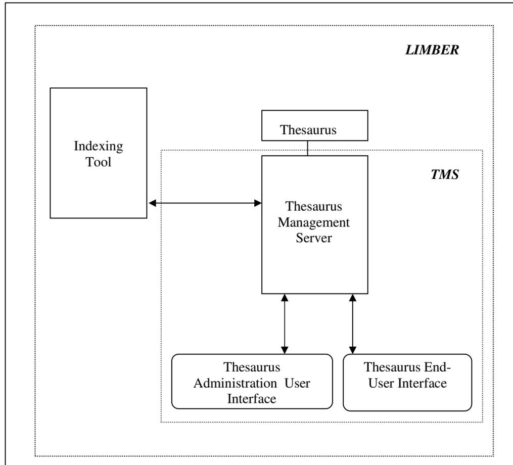
**Figure 6. LIMBER Architectural Components**
