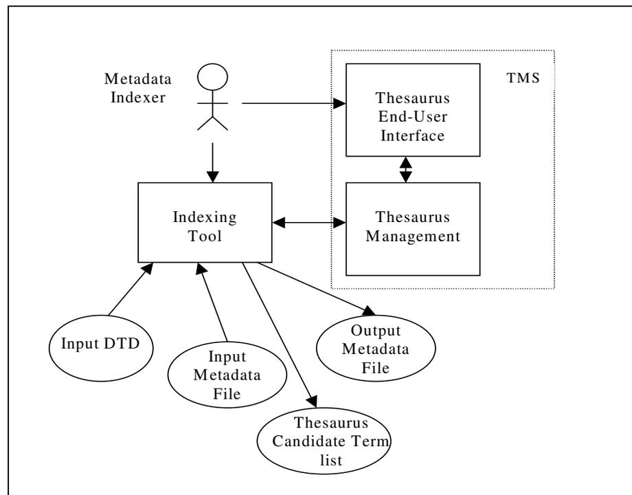
**Figure 7. Architecture of the Indexing Tool**
