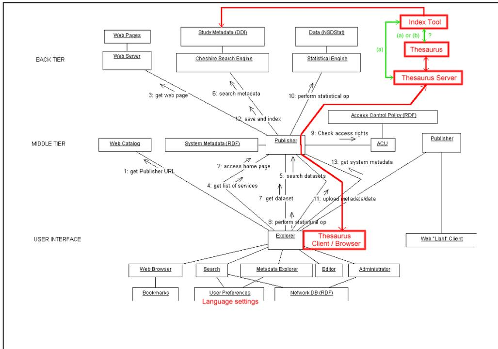
**Figure 8 Tight Integration of the Thesaurus Management System and the NESSTAR Data Archive System**
