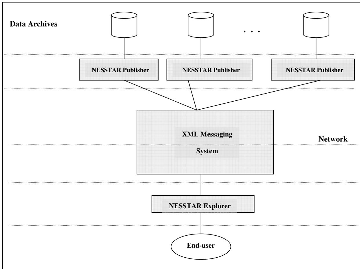
**Figure 4. NESSTAR's Distributed Architecture**
