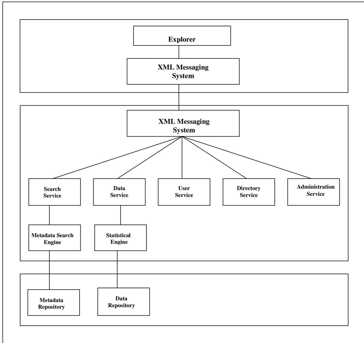
**Figure 5. NESSTAR's layered distributed architecture**
