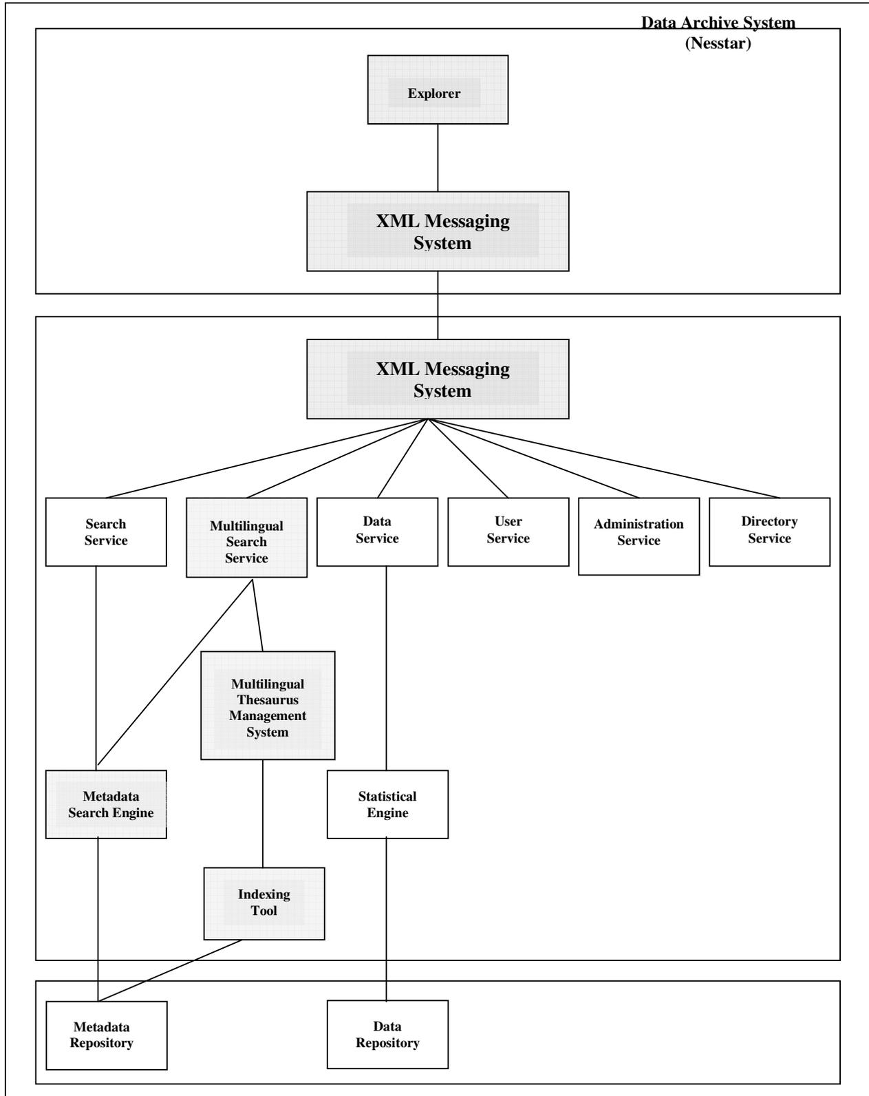
Figure 9. Tightly coupled NESSTAR/TMS integration in a layered architecture
