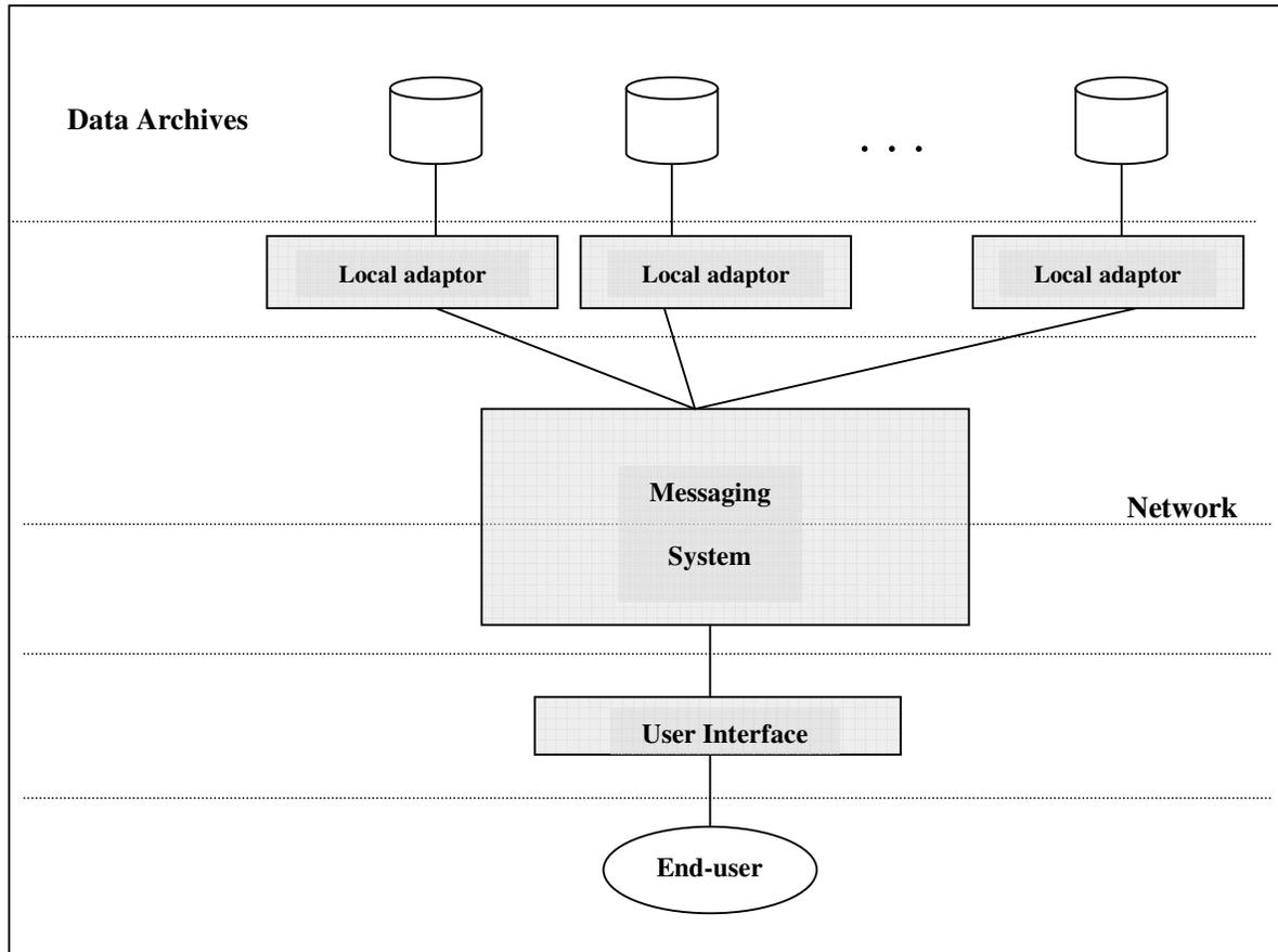
**Figure 3. A generic architecture for a distributed data archive system**
