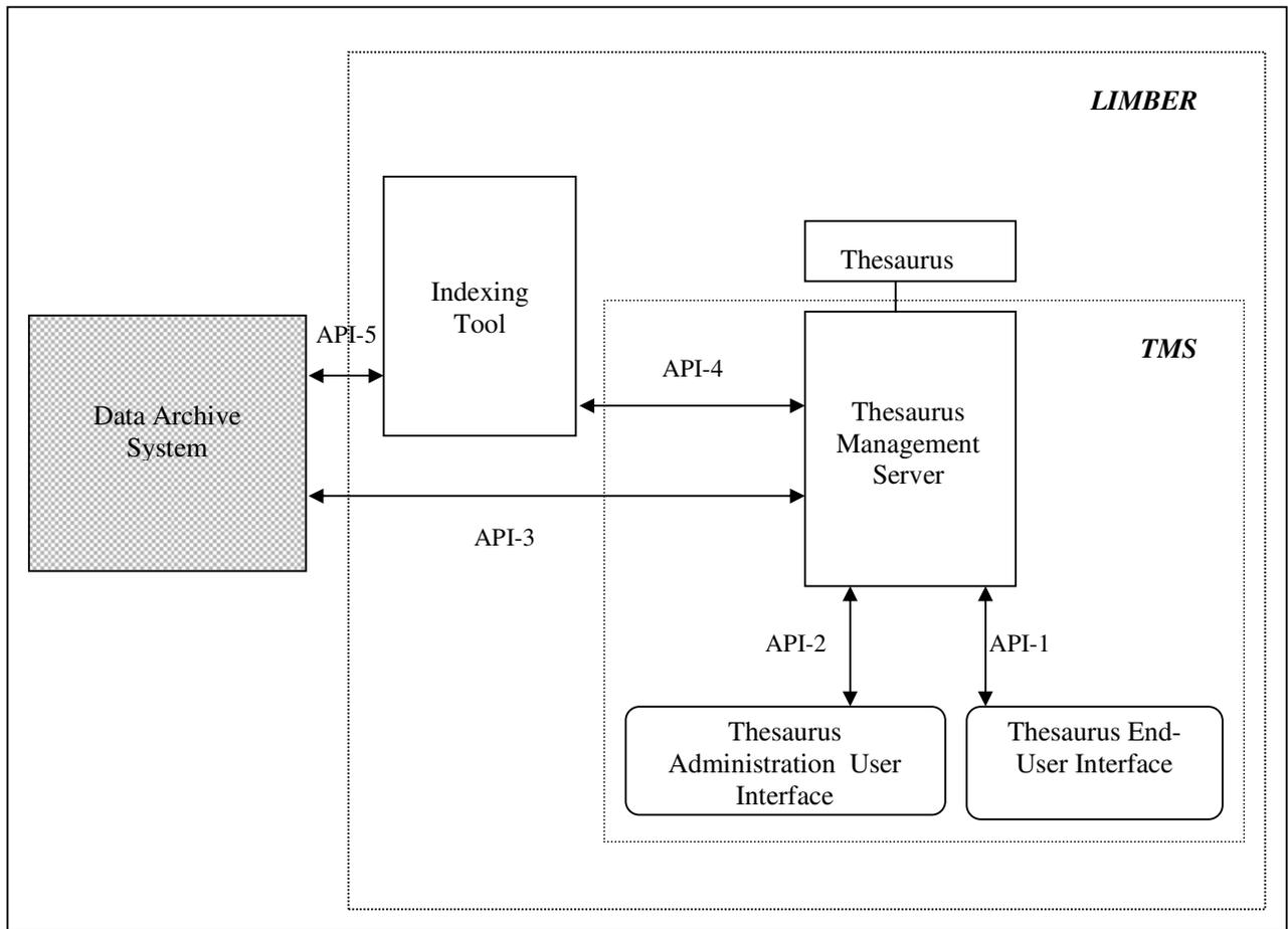
**Figure 10. Loosely coupled integration of the Thesaurus Management System and the Nesstar Data Archive System .**
