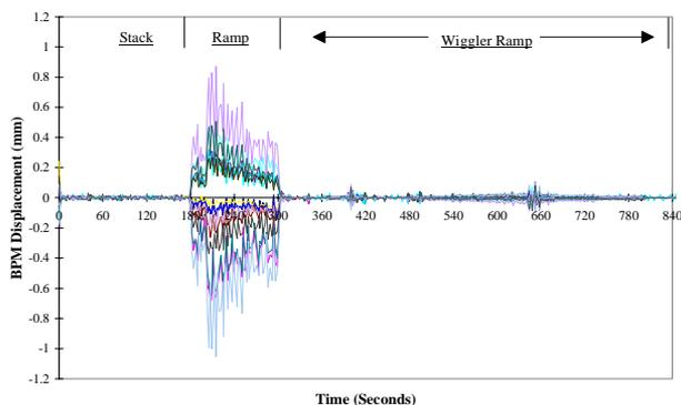
Figure 4: Vertical Orbit Control During Stacking and Ramping in HIQ
