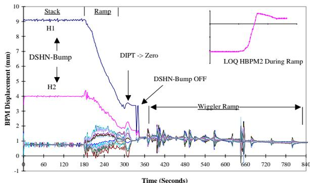
Figure 3: Horizontal Orbit Control During Stacking and Ramping in HIQ
