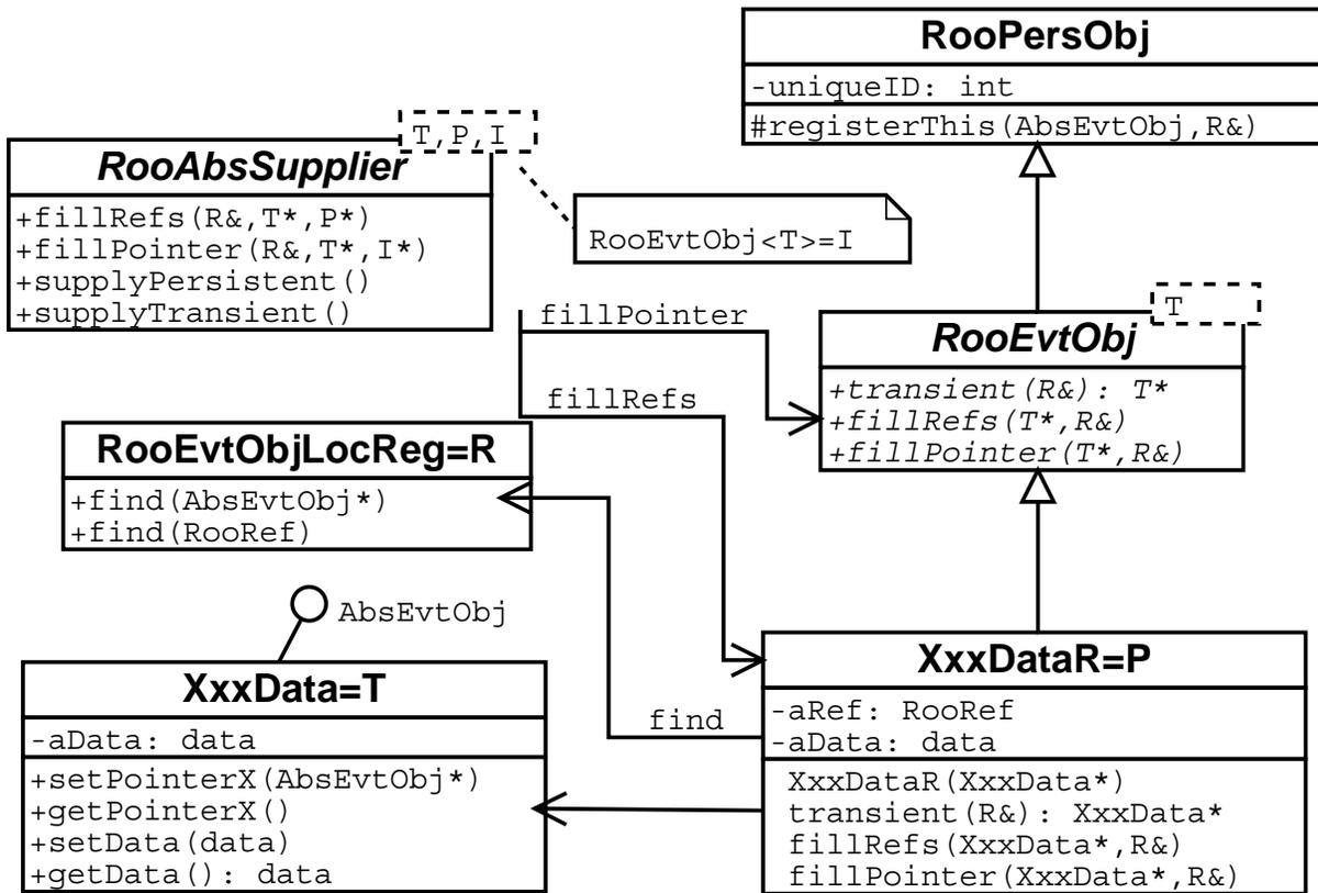
Figure 4: The figure presents an UML class diagram of the classes involved in the implementation of persistent references.
