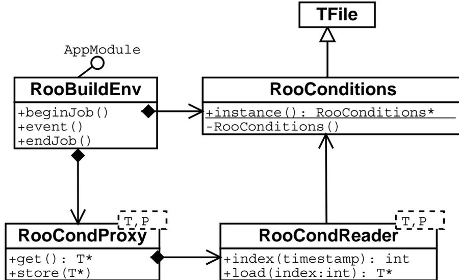
Figure 5: The figure shows an UML class diagram of the conditions data handling.
