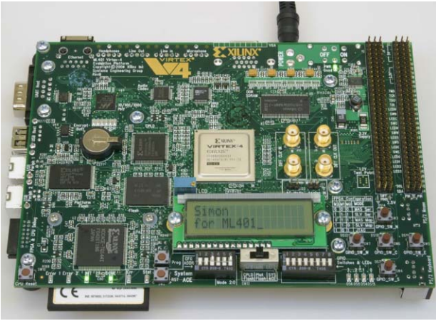
Figure 6: Xilinx Virtex4 development board.
