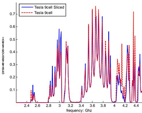
Fig 6 Zoomed in region of the generalised cascaded  $S_{21}$  matrix for a 9-cell TESLA structure comparison between an unperturbed structure and the RMS of a randomly perturbed structure for the  $TE_{11}$  mode scattered into the  $TE_{11}$  mode. Here the middle cells in the structure were randomly perturbed using slice sizes of 0mm, 1mm, 2mm and 3mm with the RMS taken for 20 different simulations.
