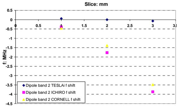
Figure 2 Frequency shifts as a function of slice size for the  $\pi$  phase mode of the second dipole band.
