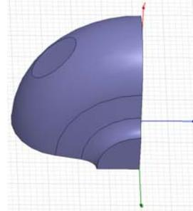
Figure 1 Isoparametric representation of a quarter of a TESLA middle cell with a 3 mm slice size perturbation applied at the equator radius.
