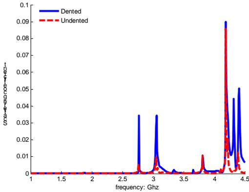
Fig. 5 Zoomed in unit cell  $S_{21}$  matrix comparison between an unperturbed structure and a perturbed structure with a slice size of 1mm for the dominant  $TE_{11}$  mode scattered into the third mode (sextupole).
