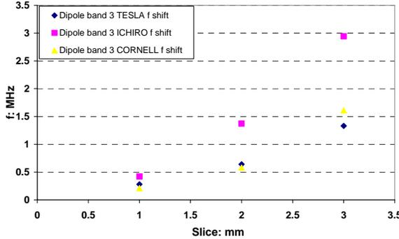
Figure 3 Frequency shifts as a function of slice size for the 0 phase mode of the third dipole band.
