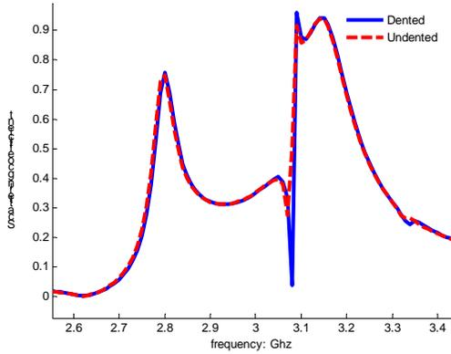
Fig. 4 Zoomed in unit cell  $S_{21}$  matrix comparison between an unperturbed structure and a perturbed structure with a slice size of 3mm for the dominant  $TE_{11}$  mode scattered into the  $TE_{11}$  mode.
