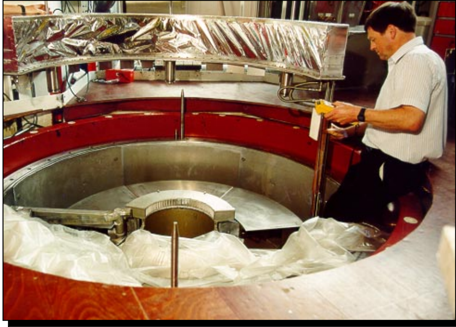
Figure 6 The graphite analyser bank being lowered into position. The entire analyser assembly, including the mounted graphite crystals, is surrounded by a nitrogen shield and fronted by an aluminium window.
