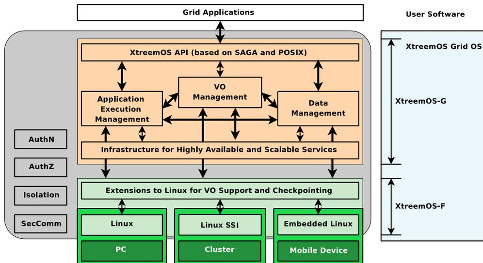
Figure 1: Layering of the XtremOS software packages.
