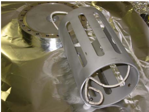
Figure 2: Stainless steel samples used for thermal outgassing and ESD tests
