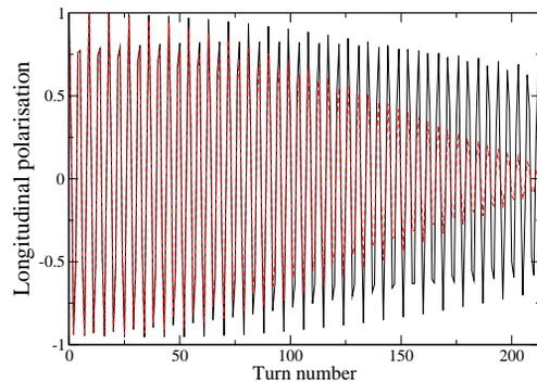
Figure 9: Depolarisation due to momentum spread of 0.5% (black solid) and 1.0% (red dash).
