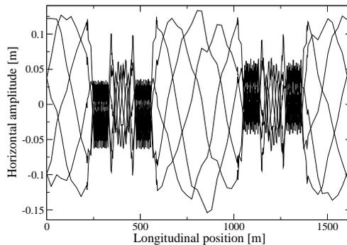
Figure 5: Horizontal beam envelope given by five particles with normalised emittance 3 Pi cm.
