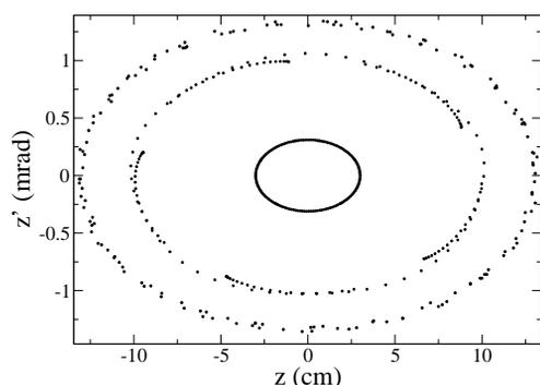
Figure 4: Vertical phase space of muons with equal emittance in the horizontal and vertical planes. The outer curve represents a 3.3 Pi cm normalised emittance.
