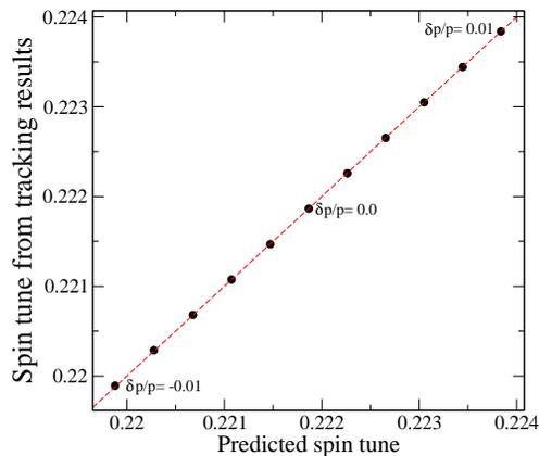
Figure 7: Predicted spin tune at momenta in the range  $\frac{\delta p}{p} = \pm 0.01$  with stepsize  $\frac{\delta p}{p} = 0.002$  compared with Zgoubi tracking result (circles). The dashed line represents equality.
