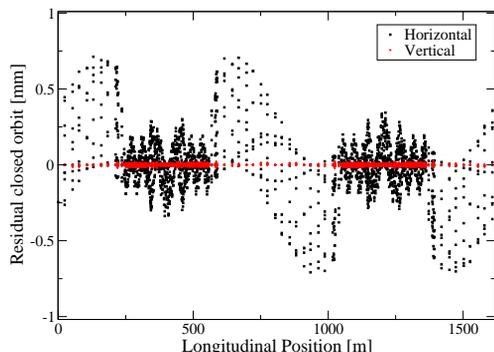
Figure 2: Horizontal and vertical residual closed orbit in the bow-tie ring calculated over ten turns. The origin is at the center of the production straight. Note the vertical scale is in the range  $\pm 1$  mm.
