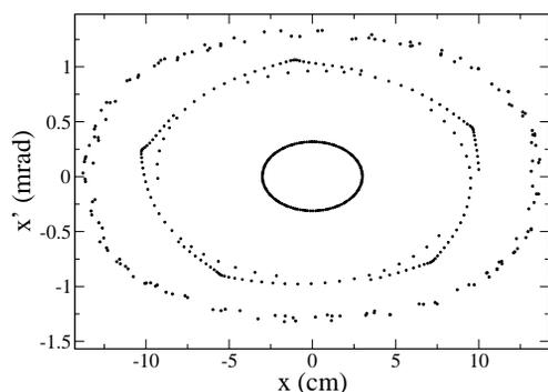
Figure 3: Horizontal phase space of muons with equal emittance in the horizontal and vertical planes. The outer curve represents a 3.3 Pi cm normalised emittance.
