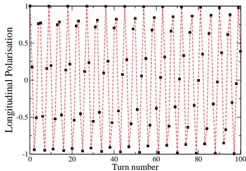
Figure 6: Longitudinal component of polarisation for muons tracked in the triangle ring (black squares) compared with spin tune prediction (red dashed).
