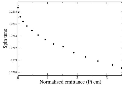
Figure 8: The variation of spin tune with transverse emittance from Zgoubi tracking results. The muons have equal emittance in the horizontal and vertical planes and are at reference momentum.
