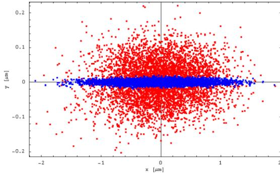
Figure 1 Beam-sizes before (red) and after tuning (blue), from a 1mrad rotation around the s-axis of QD0.
