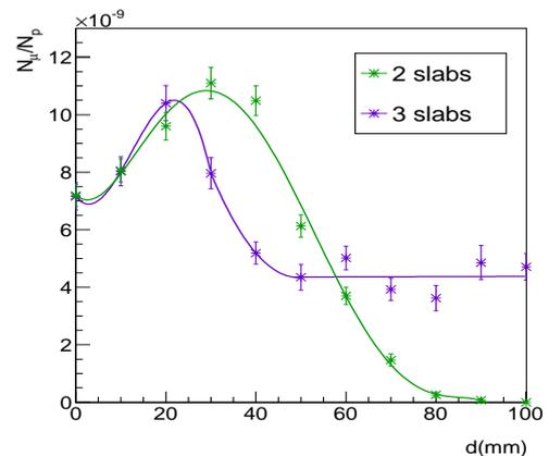
FIG. 14. Variation of the surface muon yield as a function of slab separation for a  $45^\circ$  orientation. Only muons entering the ISIS beam window are detected, and the appropriate selection cuts are applied.
