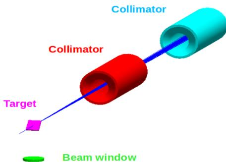
FIG. 12. GEANT4 modelling of the ISIS muon target, beam window and collimators. The target is tilted at 45 degrees and the muons produced in the target are collected by the beam window. The transmitted proton beam passes through the collimation system and impacts further on the neutron target situated 20 m downstream.
