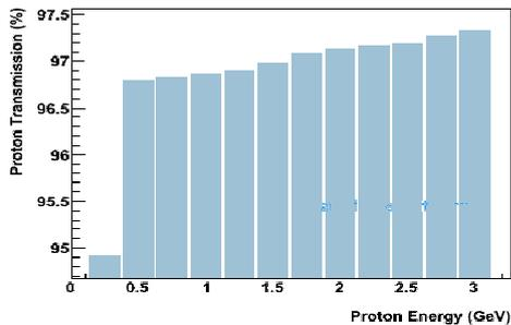
(a) Transmission through a 7 mm graphite target.
