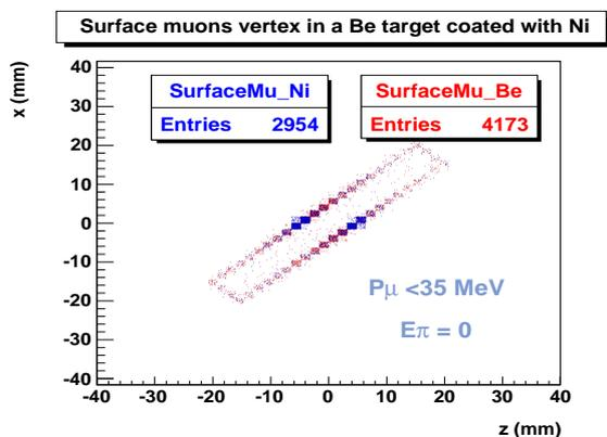
FIG. 13. Contribution of both materials to the surface muon production. Different colours represent the material in which the parent pion was produced.
