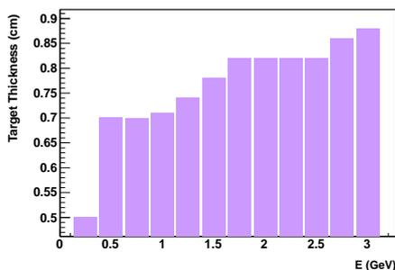
(b) Graphite target thickness for 96% proton transmission.
