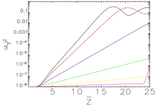
Figure 4: The effect of energy spread on harmonic lasing. The third harmonic  $|A_3|^2$  of Fig. (3) (red) is plotted for scaled Gaussian energy spreads in  $p$  of  $\sigma_p = 0.0, 0.1, 0.2, 0.3, 0.4$  and  $0.5$ . The growth rate decreases monotonically with  $\sigma_p$ . The fundamental (green of Fig. (3)) is not shown.
