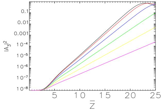
Figure 5: The effect of energy spread for a re-tuned undulator parameter of  $a_3 = 2.16$  making  $A_3$  is the fundamental. The fundamental  $|A_3|^2$  of Fig. (3) (blue) is plotted for scaled Gaussian spread in  $p$  of  $\sigma_p = 0.0, 0.1, 0.2, 0.3, 0.4$  and  $0.5$ . The growth rate decreases monotonically with  $\sigma_p$ .
