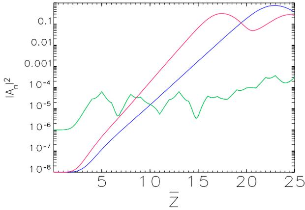
Figure 3: Scaled intensities of fundamental  $|A_1|^2$  (green) and third harmonic  $|A_3|^2$  (red) for undulator parameter  $a_1 = 4$  demonstrating the effects of relative phase changes of  $\Delta\vartheta = 2\pi/3$  at  $\bar{z} = 4, 5, 6, \dots, 24$ . For the undulator parameter re-tuned to  $a_3 = 2.16$ ,  $A_3$  is the fundamental and a separate simulation shows how  $|A_3|^2$  (blue) evolves.
