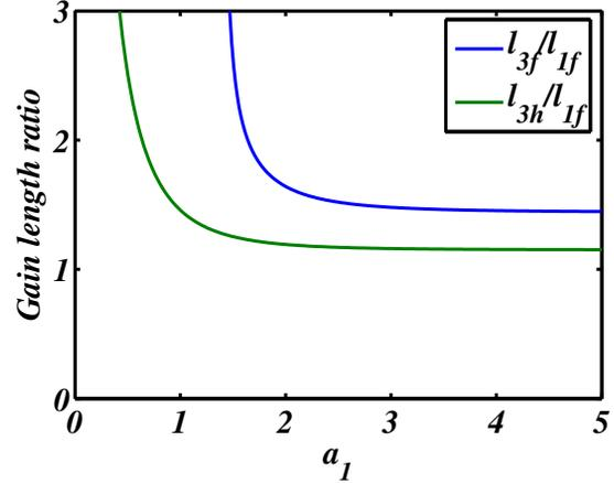
Figure 2: Comparison of gain lengths as a function of  $a_1$  for a fixed wavelength using the undulator tuned for the harmonic lasing scheme of case 1):  $l_{3h}$  (green)) and tuned for lasing at the fundamental case 2):  $l_{3f}$  (blue).
