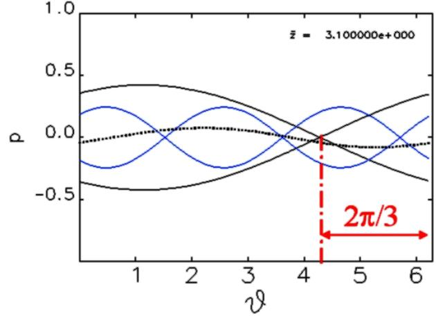
Figure 1: Schematic of electron phase space showing the fundamental separatrix (black) and 3rd harmonic separatrix (blue) following a relative phase shift of  $2\pi/3$  by both fundamental and 3rd harmonic ponderomotive potentials.
