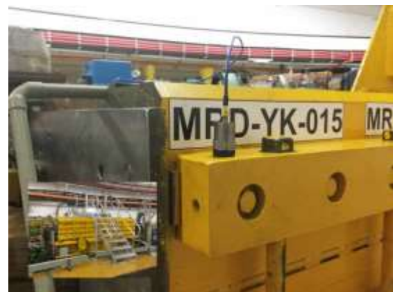
Figure 4: Vibration sensor on dipole in Synchrotron
