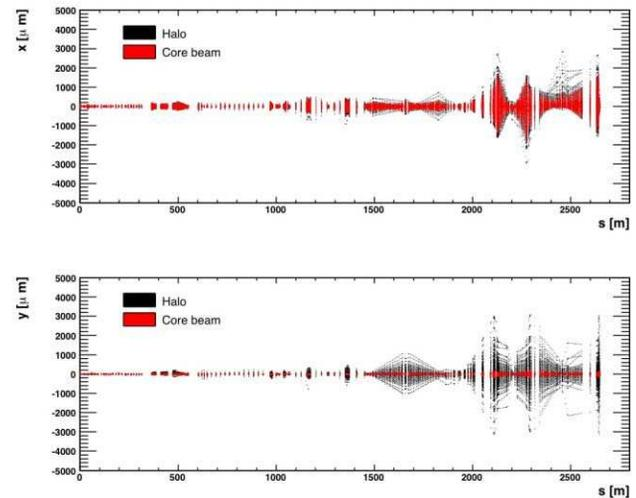
Figure 1: Tracking example for the ILC. Horizontal (top) and vertical (bottom) beam positions as function of the longitudinal coordinate  $s$  in the BDS. Halo particles are shown in black and core beam particles in red.
