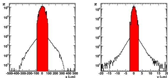
Figure 2: Transverse beam profiles at the BDS entrance.
