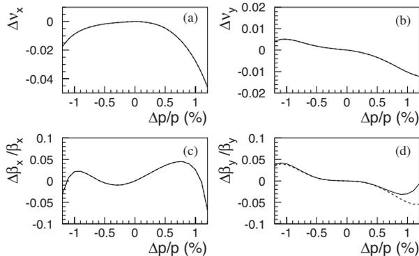
Figure 4: Chromatic effects for the HER ring. Betatron tunes (upper) and  $\beta$  functions (lower) as a function of momentum deviation in the horizontal and the vertical plane. The solid and dashed lines show the case in which the sextupole magnets for the *crab waist* on and off, respectively.
