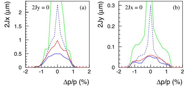
Figure 5: Horizontal aperture (a) and vertical aperture (b) as a function of momentum deviation. Green and blue solid lines show the sextupole magnets for the *crab waist* are turned off and on, respectively. Further octupole corrections are indicated by red solid lines. Blue dashed lines show the case without fringe effects for the *crab waist* on, while octupole corrections off.
