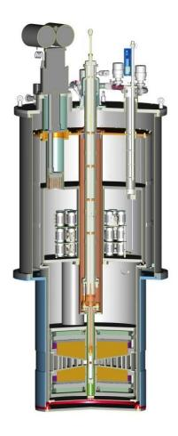
Fig. 1 The 14T superconducting magnet in a cryostat with helium re-condensed by PTR (by courtesy of Oxford Instruments)
