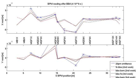
Figure 2: Monitoring of the position reading after BBA
