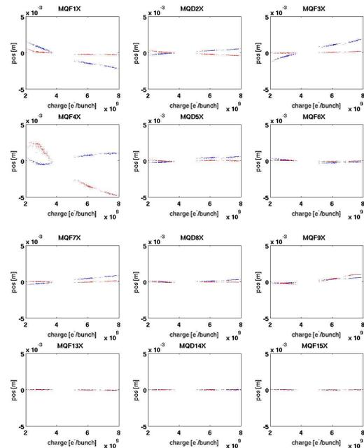
Figure 1: Horizontal (blue) and vertical (red) position readings as function of intensity ( $e^-$  per bunch) in the 12 striplines BPMs installed in the EXT.
