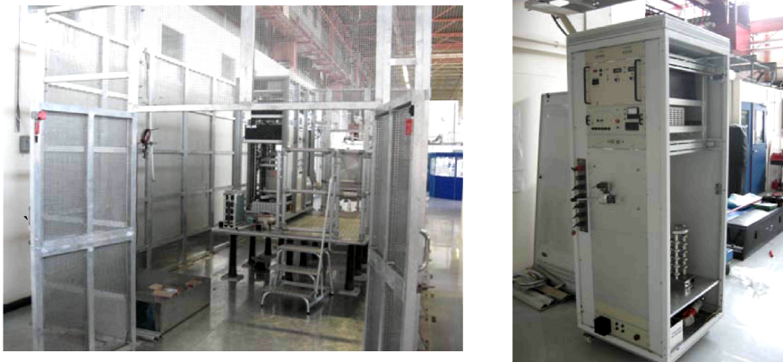
FIGURE 9: The high voltage cage and platform and the 70 kV DC power supply.
