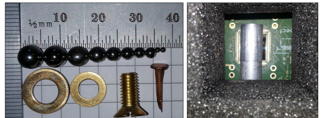
Fig 11. LEFT: A photograph of the objects measured, with scale shown. RIGHT: GP2 with aluminum sample holder in front. \text{B}_4\text{C} collimation is seen framing the picture, placed to reduce background from air scatter. All objects shown on left were placed inside the sample holder and held in place with aluminum foil.
