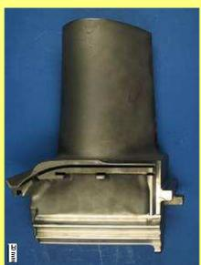
The blade was positioned within the beam with the SScanSS program
