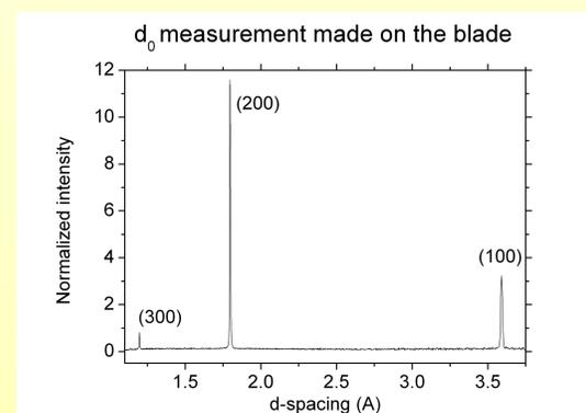
Diffraction pattern showing the **(100)/(300) superlattice reflections and the (200) reflection**, where diffraction peaks of both phases are overlapping.
