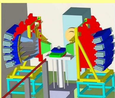
**ENGIN-X (ISIS):** Time-Of-Flight neutron diffractometer
