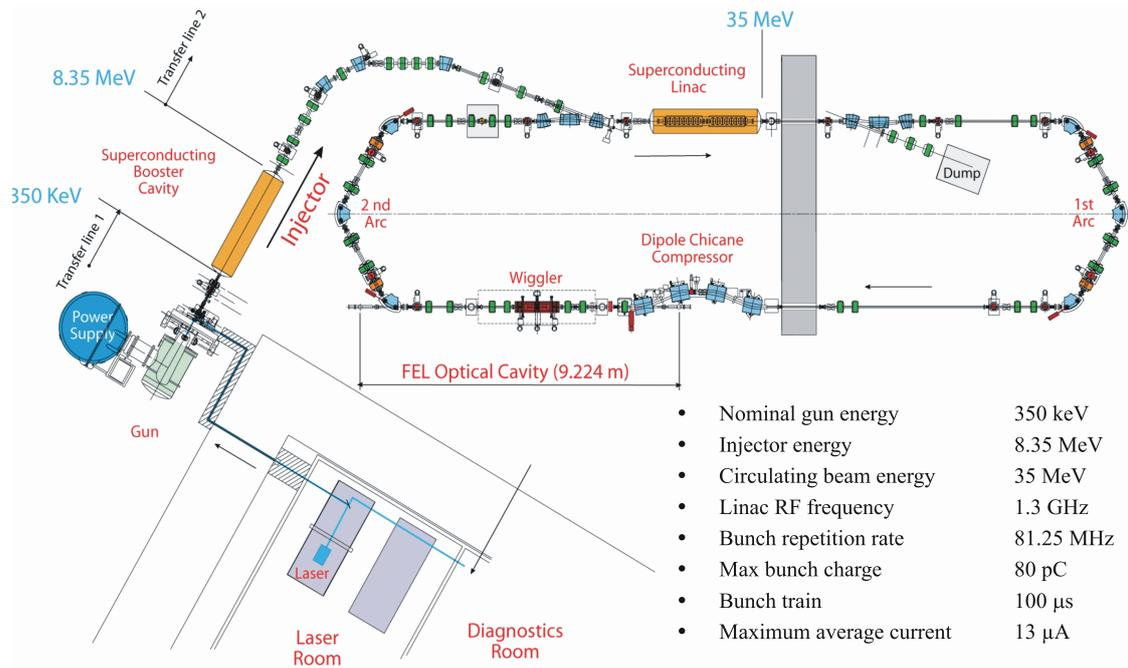
**FIGURE 1.** Schematic showing the layout of the ALICE machine and its main parameters.
