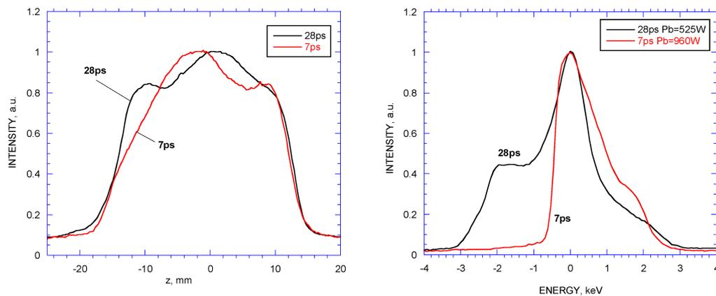
**FIGURE 4.** (Left) Bunch length with 7 and 28 ps laser pulses (Right) Compensated energy spread
