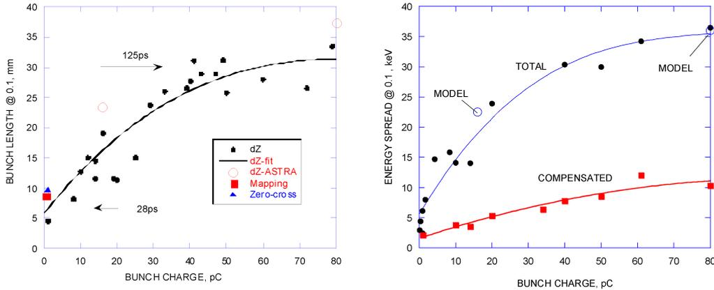
FIGURE 2. (Left) Bunch length at 10% of peak (Right) Total and tilt-compensated energy spread
