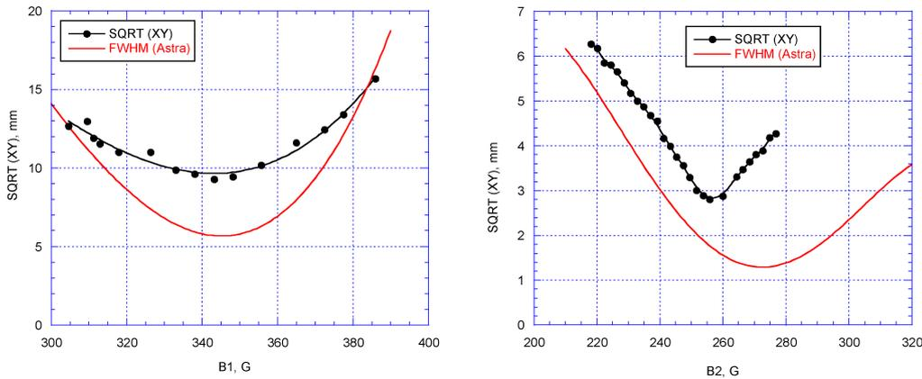
FIGURE 3. (Left) Beam size at the 1<sup>st</sup> solenoid (Right) Beam size at the 2<sup>nd</sup> solenoid
