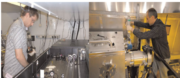
Fig. 3. (Color online) Installation of the multi-pass power amplifier (left) and the chirped pulse compressor (right).
