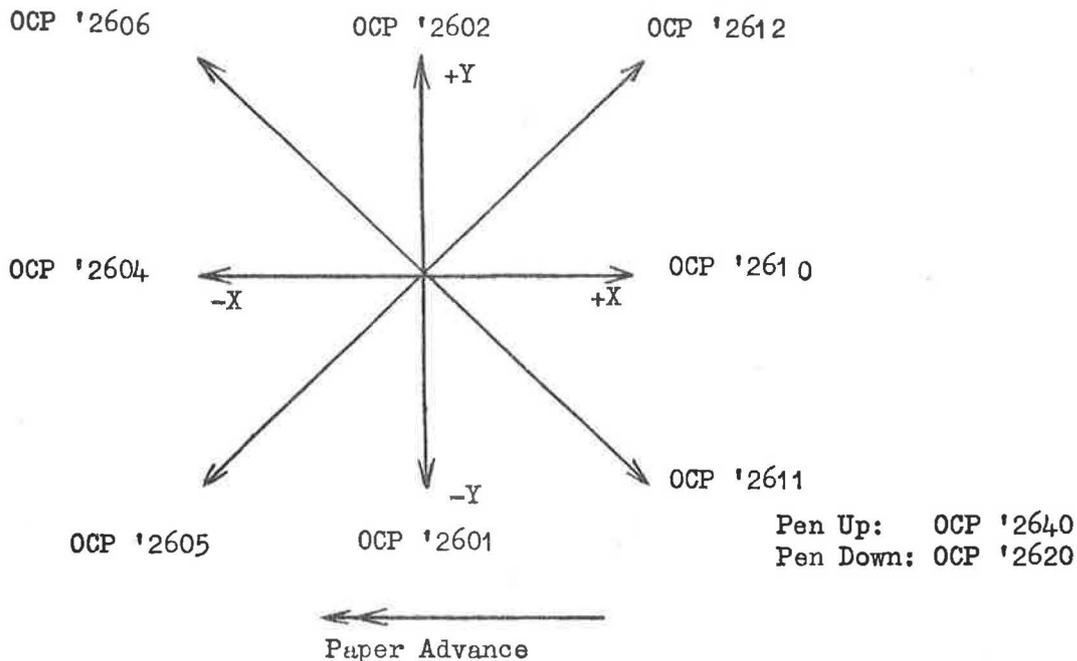
To synchronize the OCP's with the operation of the plotter, the following SKS is provided.
