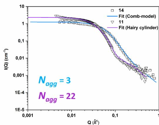
Figure 3: SANS data and fits of A) conjugate **14** (CP(PPEGA)<sub>10</sub>)<sub>2</sub>,  $10 \text{ mg mL}^{-1}$  in  $D_2O$  and B) conjugate **11** (CP(PEG)<sub>2</sub>,  $10 \text{ mg mL}^{-1}$ ) in  $D_2O$ .
