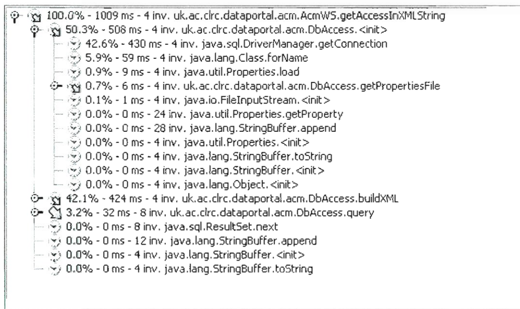
Figure 14: JProfiler examples of CPU usage on a Data Portal module.
