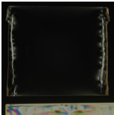
Figure 3. Stress free slice of Yb:YAG crystal. Picture taken under crossed polarizers, size 100\*120 mm.
