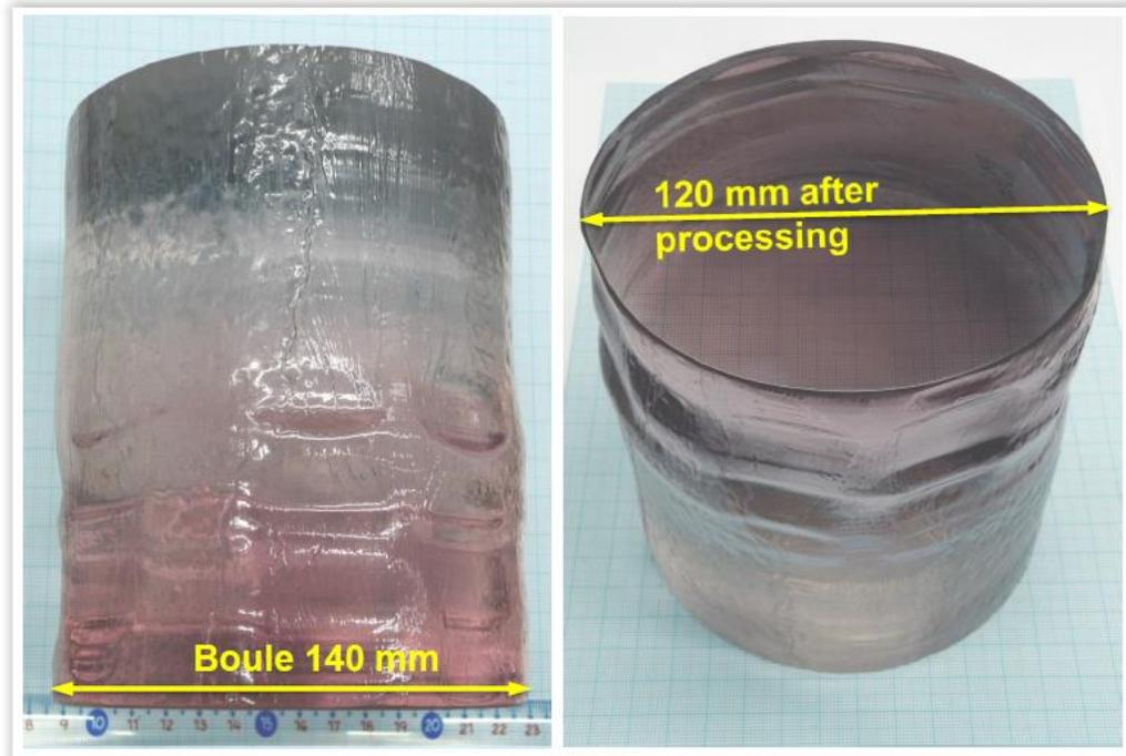
Figure 2. Yb:YAG laser quality monocrystals.
