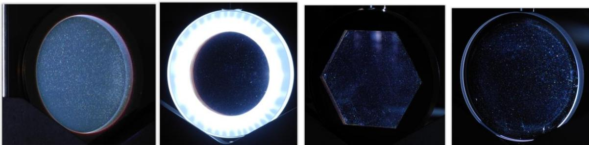
Figure 5. Yb:YAG laser slabs ( $\phi 55 \times 5$  mm) under inspection with bright light. (From left to right) Yb:YAG-Cr:YAG co-sintered ceramic slab from Konoshima company; monocrystalline slab with ASE structure from Crytur; monocrystalline slab with hexagonal Cr:YAG cladding from Crytur; plain monocrystalline slab from Crytur
