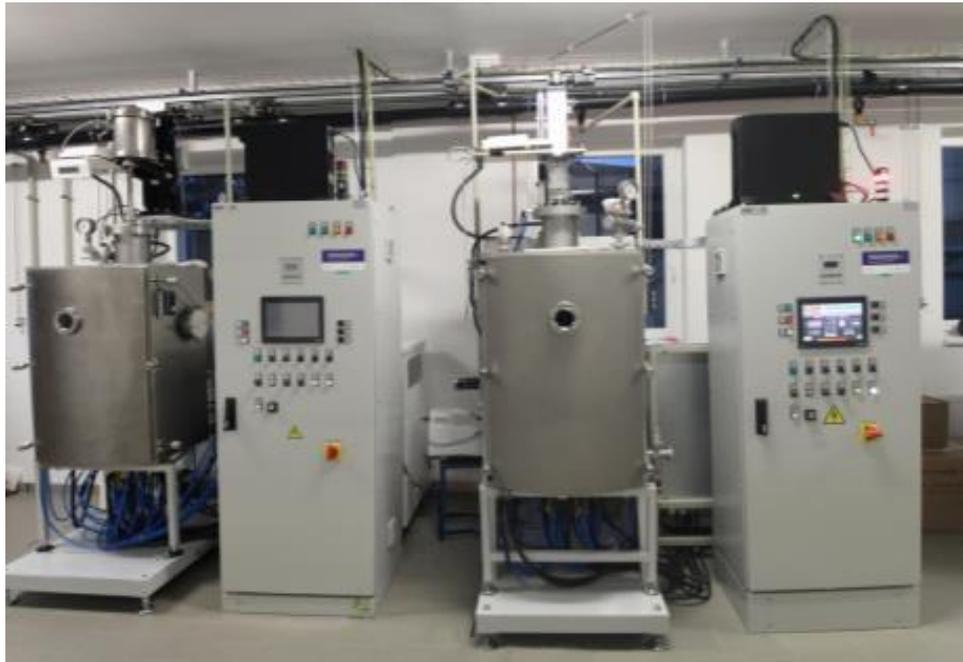
Figure 1. Crystal growth pullers built by Crytur Ltd..
