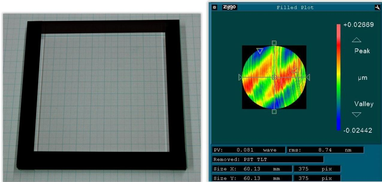
Figure 4. (left) Picture of Cr:YAG cladded monocrystalline Yb:YAG laser slab of size 120x120 mm. (right) Result of the transmitted wavelength distortion measurement of the element, used wavelength 633 nm.
