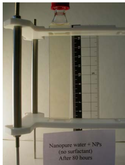
Figure SI-5 Long-term Stability of the SiO 2 NP Dispersions. Unfunctionalised SiO 2 NPs dispersed in nanopure water after approximately 80 hours.
