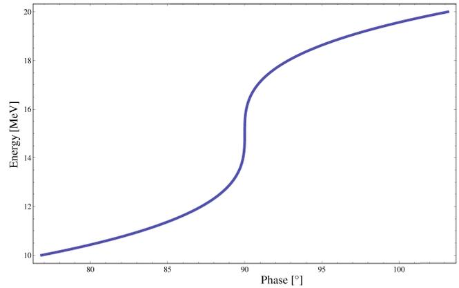
Fig. 4: An example of the so-called serpentine acceleration for the EMMA ring for the central trajectory, where the longitudinal  $H_0 = 0$ . The harmonic number is assumed to be 11, with the RF wavelength 0.405m. The parameter  $a$  from Eq. (103) is taken to be  $2.686310^{-5}$ .
