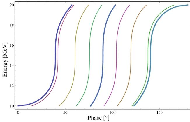
Fig. 5: Examples of serpentine acceleration for the EMMA ring, with varying value of the longitudinal Hamiltonian. The limits of stability are given at values of the longitudinal Hamiltonian of  $\pm 0.31272$ , corresponding to either a 0 phase at 10MeV, or a  $\pi$  phase at 20MeV.
