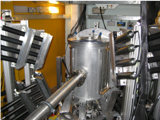
Figure 3.1: The VESUVIO Spectrometer at the ISIS Pulsed Neutron and Muon Source
