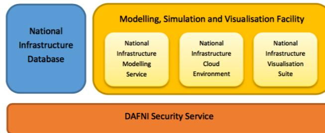
Figure. 1. DAFNI Core Capabilities. Cloud, modelling and visualisation services are grouped into a Modelling, Simulation and Visualisation facility
