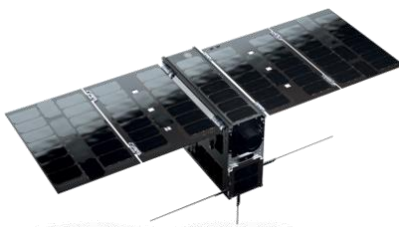
Figure 1-1: 6U EPIC platform by AAC Clyde Space. It offers a 4.5U payload volume, a 120 W peak payload power, and a pointing stability of 7.2 arcsec. On a larger 12U platform it is possible to double payload volume and power.
