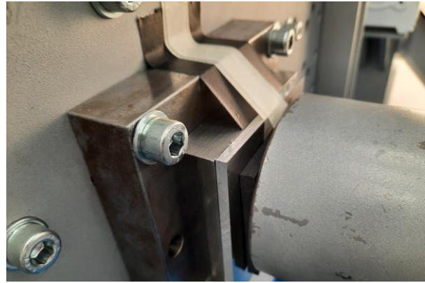
Figure 3 Detail of the impact point showing from left to right, reverberant plate, bolted anvil, semi-sacrificial steel plate, aluminium plate and rubber layer.
