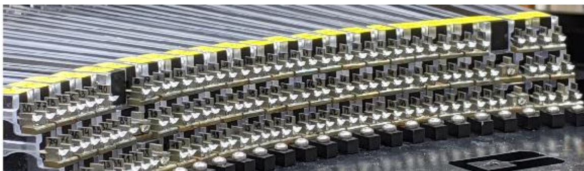
Figure 7. MOS, mIFU guide buttons positioned on the retractors at the edge of plate B.
