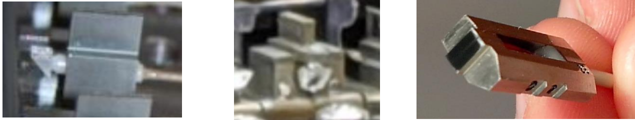
Figure 1. MOS button assembly with its 1.5 mm prism on the test bench (left), mIFU button assembly with its 2 mm prism located under the lens holder on its retractor (center) and MOS slitlet during inspection with its 24 fibres (right).
