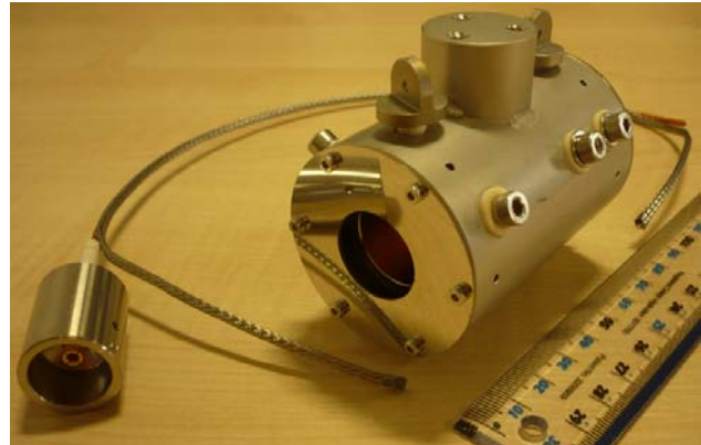
Figure 4: Assembled Faraday cup together with a double shielded cable equipped with a floating shield connector.
