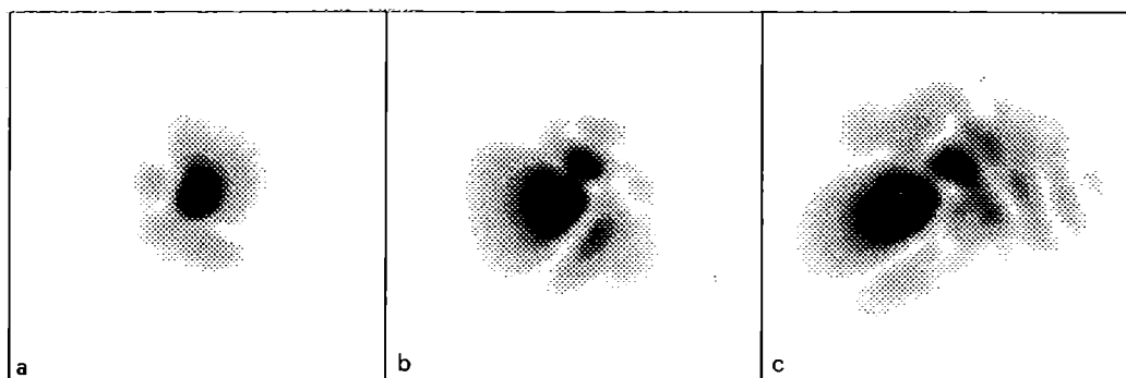
Fig.2: Simulation of realistic beams, the amplitude of the phase "disturb" increases from (a) to (c).
