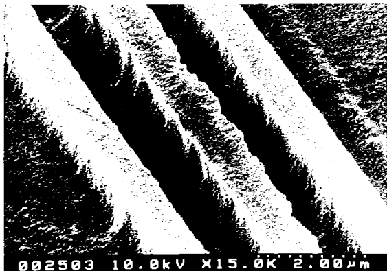
Figure 3. SEM images of X-ray mask showing 1.2 micron lines and 0.7 micron spaces as well as imperfections. (a) along the walls of the gold lines (b) at the end of the gold lines.
